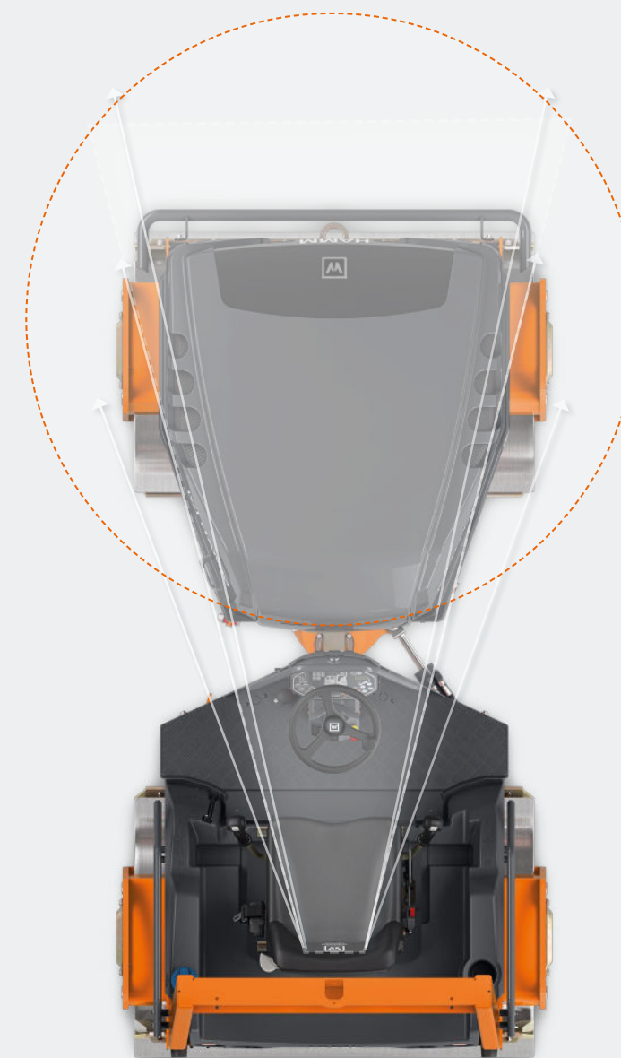
Clear view of the drum edges - thanks to the wasp waist!
